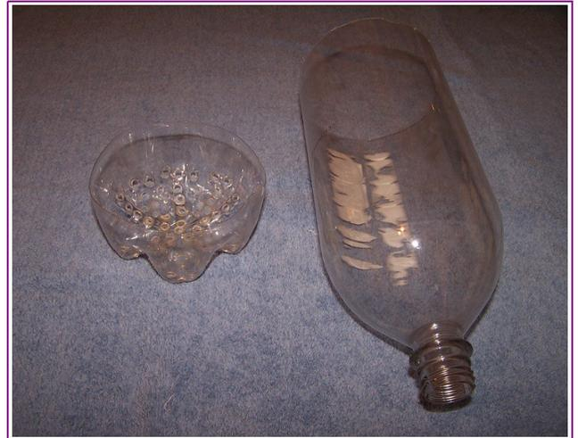
Now grind off enough of the threads from the neck of the bottle so they fit inside the  $\frac{3}{4}$  inch straight PVC tubing connectors. Once they fit inside, then glue them in place using the epoxy glue or hot glue. Try and make them as straight as you can so the bottles point straight up (it looks better when they are all straight).
