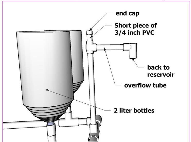
The picture to the left shows the overflow tube going straight down into the reservoir. The reservoir in the picture hasn't been painted yet. But like you did with the 2 liter bottles, you'll want to paint the outside of your reservoir black to light proof it, then white to reflect light.
