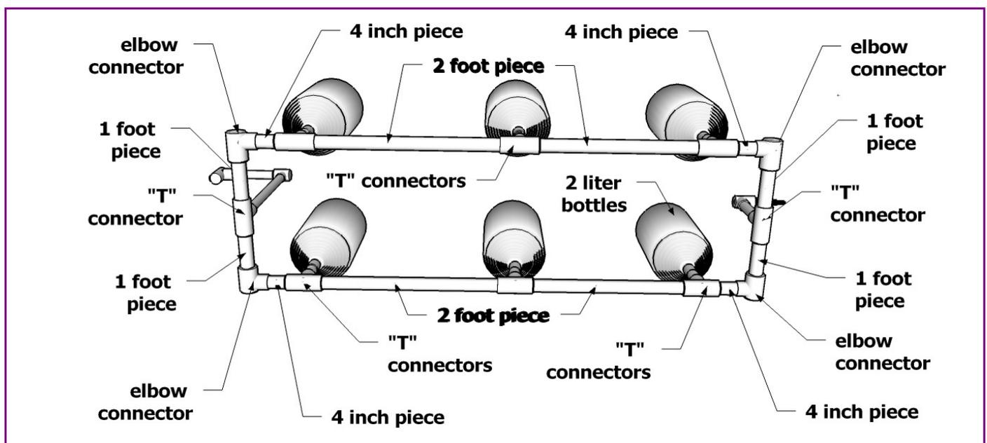
The image below is a top view of the base of the hydroponic system. Notice The short pieces of  $\frac{3}{4}$  inch PVC tubing pointing straight up from each of the “T” connectors where each of the six 2 liter bottles will be placed. Make sure these pieces aren’t too long or the 2 liter bottles can become a bit tipsy. Two to three inches should be fine, and again make sure to dry fit everything together first before gluing them together.
